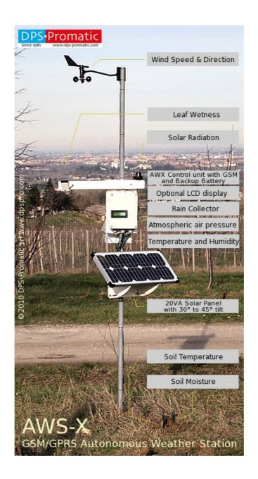
AWS-X GSM/GPRS weather station
